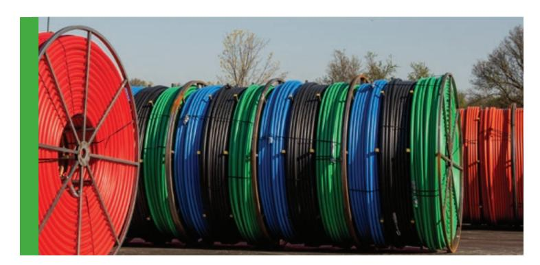
Atkore's Comm-Line is one of the most common conduit solutions for telecommunications and fiberoptic projects across the United States. It is available in IPS (Iron Pipe Size) in diameters from ¾ to 16 inches and DIPS (Ductile Iron Pipe Size) in diameters 4 inches and up. It can be installed in existing conduit or via plow, direct burial or HDD (horizontal directional drilling) installation methods.
